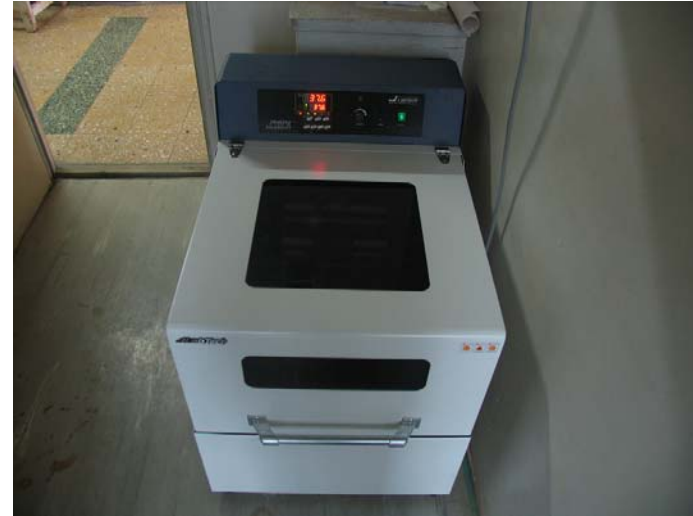
Incubator (temperature range 5 – 60°C)
